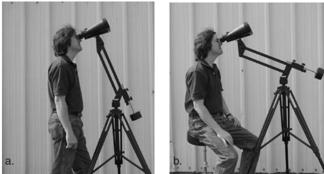
Figure 5. The binocular will remain on target as you adjust the height using the parallelogram. The standing person in (a) is looking at the same thing while seated in (b). Note that only the parallelogram has moved; the tilt angle of the binocular has not. The pivot disk and binocular altitude should not be adjusted for this feature to work.
