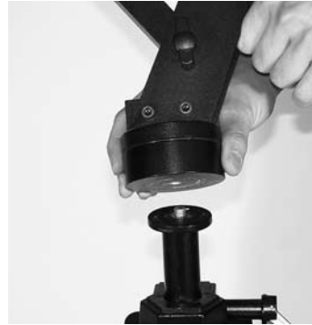
Figure 2. Line up the threaded pan head attachment shaft of the tripod with the threaded hole on the bottom of the pivot disk. Then hold the binocular mount still while turning the pivot disk to thread it onto the shaft.
