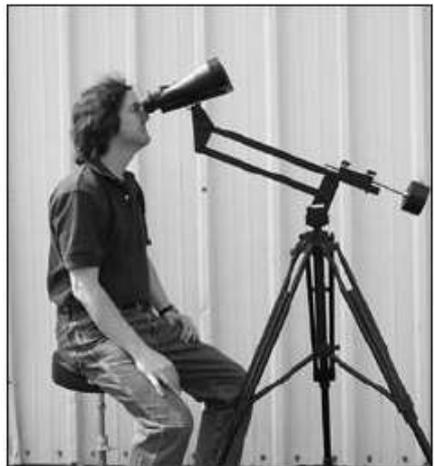
**Parallelogram Safety Stop:** The parallelogram has a safety stop to prevent the aluminum bars from completely collapsing. This ensures that no fingers will be caught and crushed by an accidental fast closing of the parallelogram. This feature will also prevent the counterweight from hitting the tripod.
